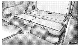
**Flat Load Floor**Unsnap the flipper panels on the third row seats and flip them forward on the back(s) of the second row seat(s).
